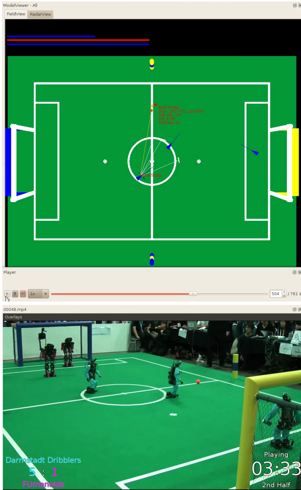
Fig. 3: Model viewer showing the robots' and ball's positions (top) synchronized with the external camera image (bottom) including some overlays generated from the logged data.
