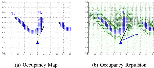
Fig. 9: Modifying the initial trajectory (Dashed arrow) of the robot based on a potential field to avoid obstacles (solid arrow)
