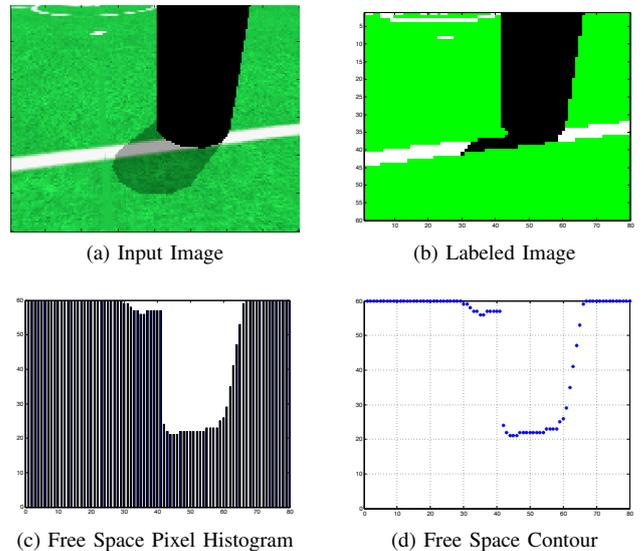
Fig. 5: Pixel Histogram based Free space Detection
