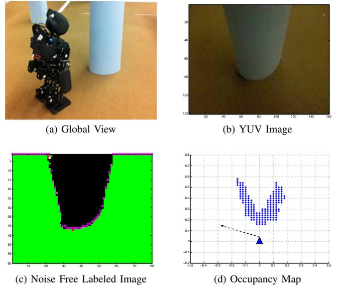
Fig. 8: The full pipeline of the occupancy grid system including contour detection.
