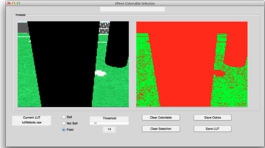
Fig. 3: Human interface for labeling pixels as color classes. Green pixels are ground and red pixels are unclassified.
