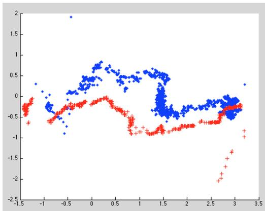
Fig. 13: Path comparison between simulation (blue) and real hardware (red) when starting from the center, where the coordinates are measured in meters and the goal is (3,0)
