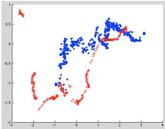
Fig. 12: Path comparison between simulation (blue) and real hardware (red) when starting from the right, where the coordinates are measured in meters and the goal is (3,0)
