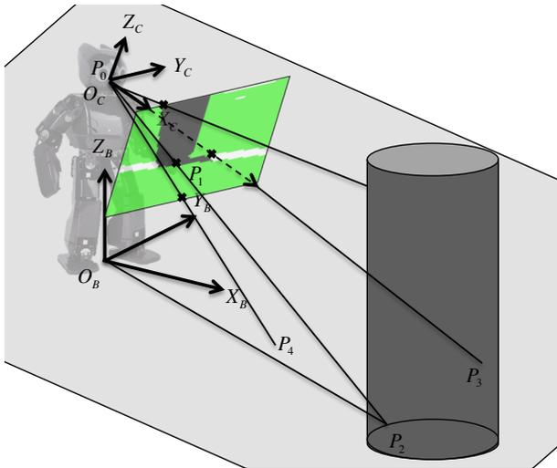
Fig. 7: Projective Transformation Schematic
