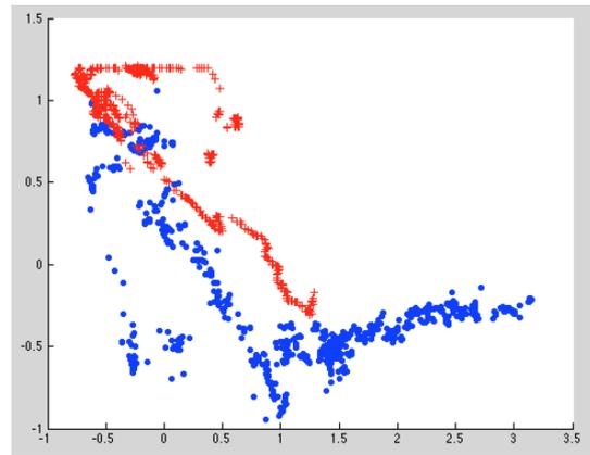
Fig. 11: Path comparison between simulation (blue) and real hardware (red) when starting from the left, where the coordinates are measured in meters and the goal is (3,0)
