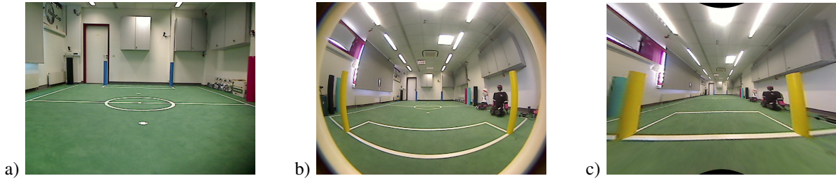
Fig. 5. Wide-angle lens: a) A raw camera image of a RoboCup soccer field without the wide-angle lens. b) An image from the same perspective using the wide-angle lens shows the increased field of view and the introduced barrel distortion. c) Undistorted camera image computed using Eq. 1.
