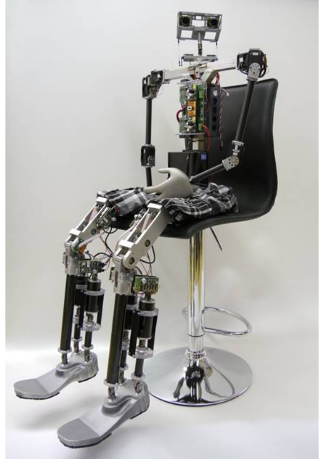
Fig. 12. Design prototype of Sweaty II - not yet optimized for light weight
